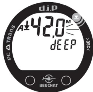
Fig. 64 - SET MAX DEPTH ALARM
