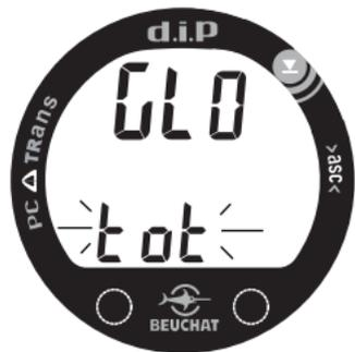
Fig. 66B - SET NAV BACKLIGHT MODE (TIME OUT)
