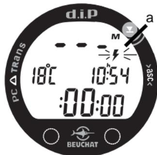
Fig. 6 - LOW BATTERY (ACTIVATION)
