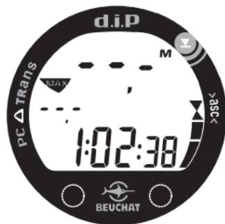
Fig. 41 -MAX OPERATING DEPTH EXCEEDED
