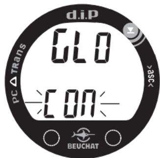
Fig. 66A - SET NAV BACKLIGHT MODE (CONSTANT)
